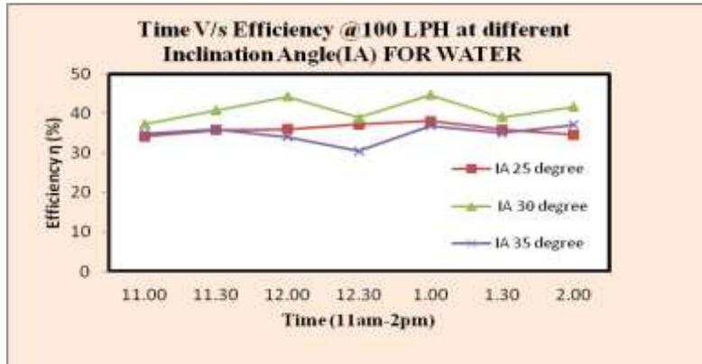
Variation of instantaneous collector efficiency with time at different inclination angle and mass flow rate of 0.02778 kg/sec for water
