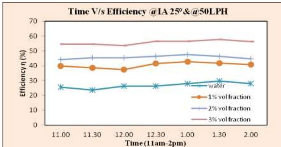
Variation of instantaneous collector efficiency with time for 25° inclination angle and mass flow rate of 0.01389 kg/sec.
