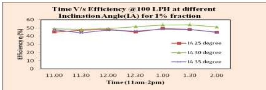
An experimental study has been carried out to investigate the efficiency of solar flat plate collector using BN/H<sub>2</sub>O nanofluid. The volume concentration of BN/H<sub>2</sub>O nanofluid has been varied from 1 % to 3 %. The performance of solar flat plate collector was evaluated at different inclination angle. The effect of mass flow rate on the performance of solar flat plate collector has also been investigated.
